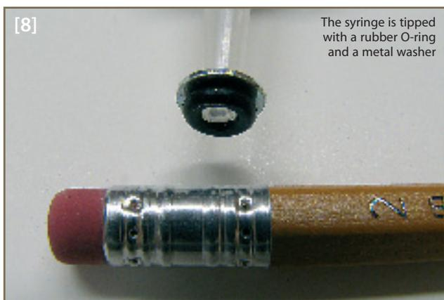
The syringe is tipped with a rubber O-ring and a metal washer
