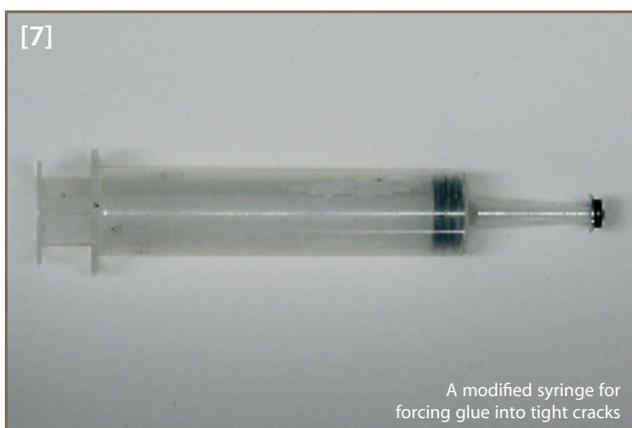
A modified syringe for forcing glue into tight cracks
