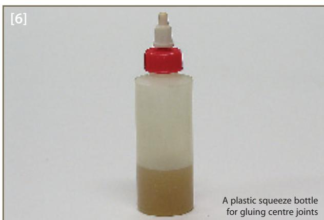
A plastic squeeze bottle for gluing centre joints
